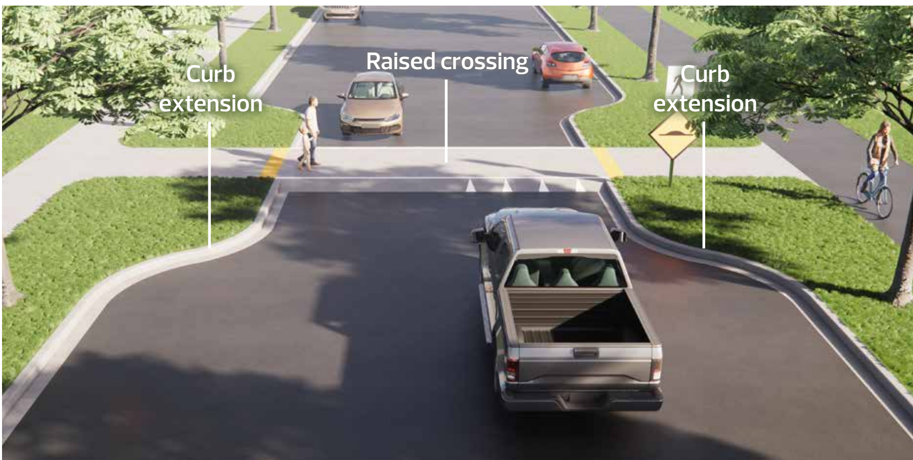
Example of raised crossing with curb extensions
